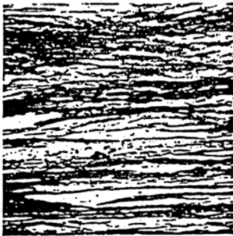
Figure 2: Unheated Bedspring Material. The Metal Consists of Radically Elongated Grains of Pearlite (Dark) and Ferrite (Light) Grains. Nital Etch. 500X.
