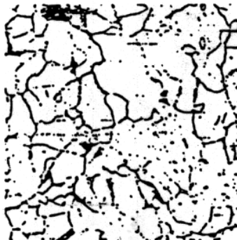
Figure 5: Bedspring Material Heated to 1,800°F for 2.5 Hours and Air Cooled. Because of Decarburization, the Material Now Consists Entirely of Recrystallized Ferrite Grains. Nital Etch. 500X.
